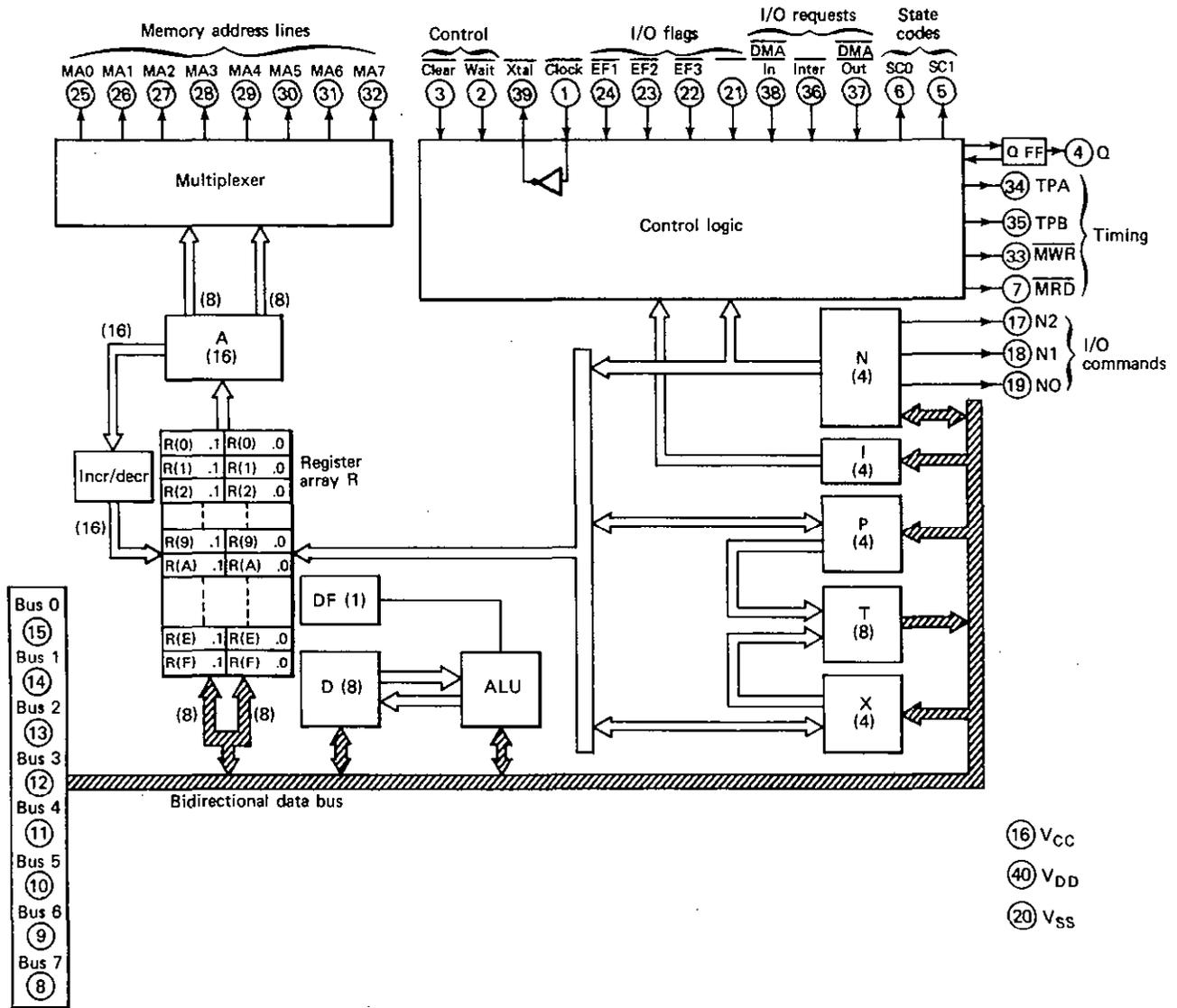
Fig. 7 Microstructure of the CDP 1802.
