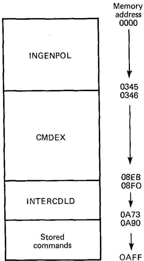
Fig. 12 MAGSAT command firmware.
