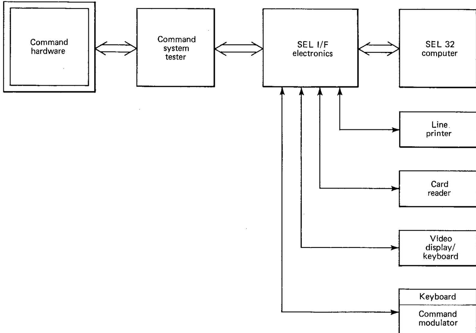
Fig. 13 Command system test configuration.
