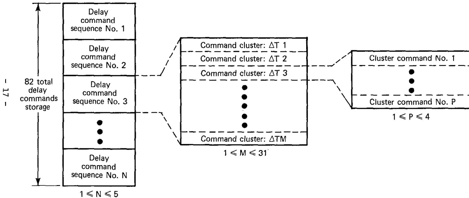
Fig. 5 Delayed commands RAM space allocation.
