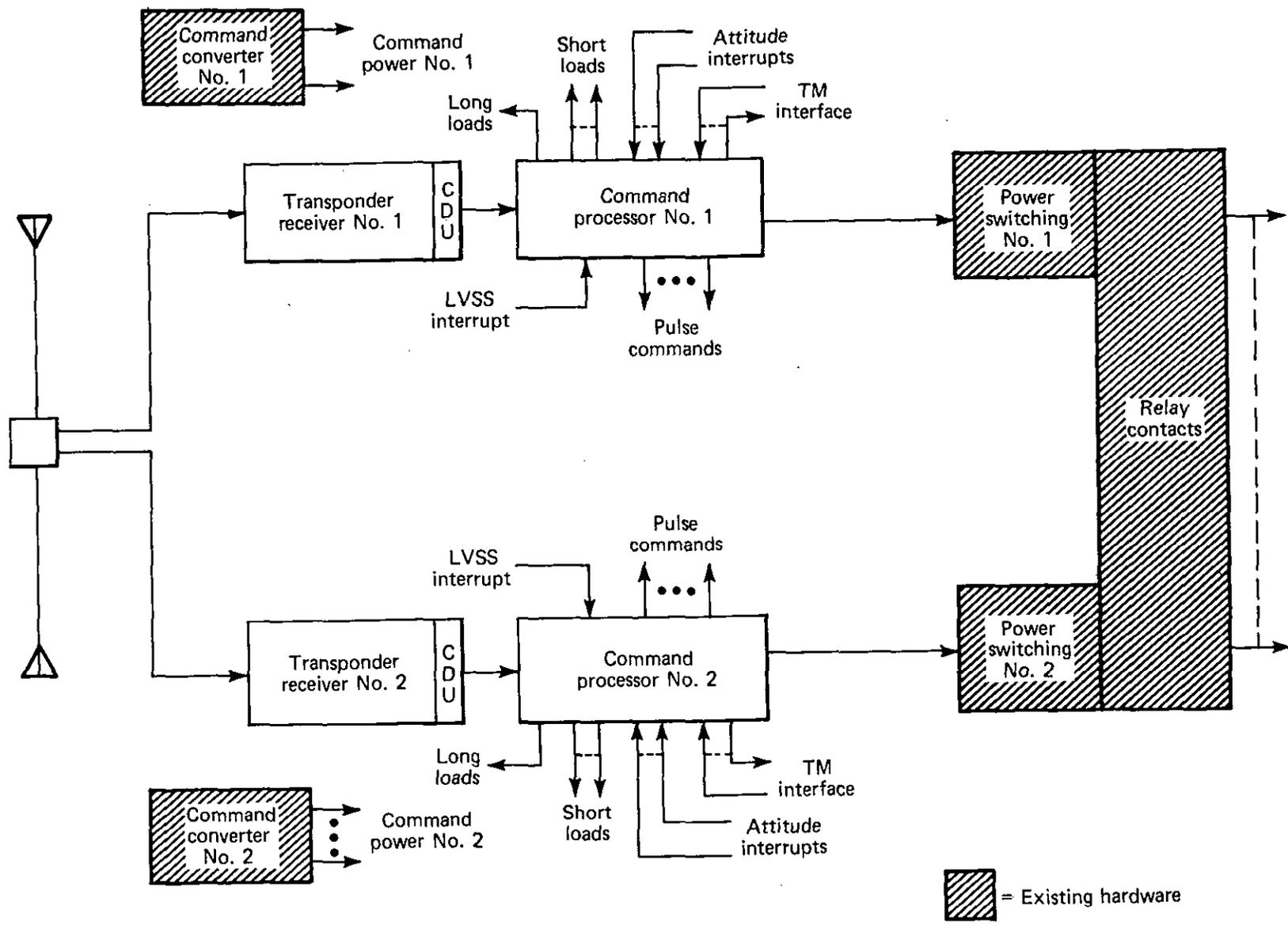
Fig. 2 MAGSAT command subsystem.
