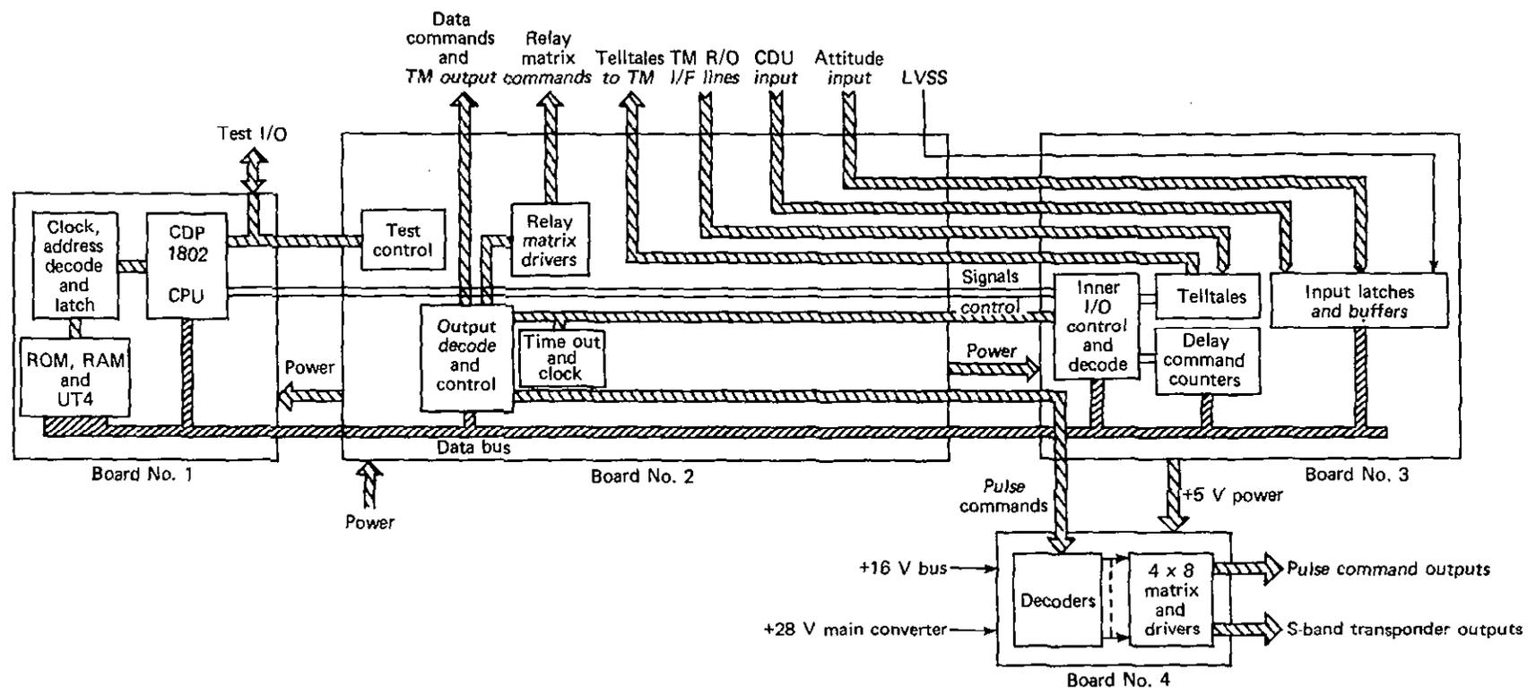
Fig. 9 Block diagram of MAGSAT command processor flight boards.
